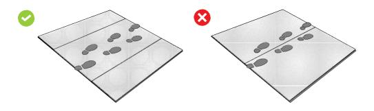
For Coral duo (Everfort vinyl backing) multiple width application, trim from the top with a straight edge and knife. Remove the 2.5cm edge border from all edges and any further material as necessary to maintain a continuous rib design between sheets.
